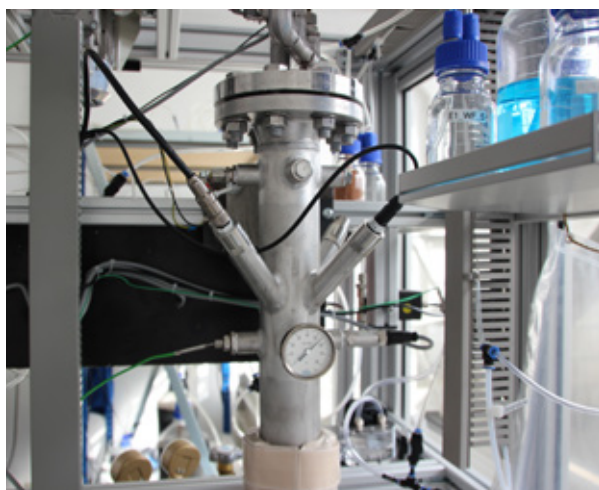
Methanation test rig.
