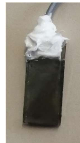
Dark colored electrode after measurement due to Cu 0
