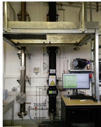
Laboratory equipment: bubble column and batch reactors © DBI-Gruppe
