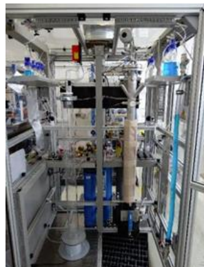
Laboratory equipment: bubble column and batch reactors © DBI-Gruppe
