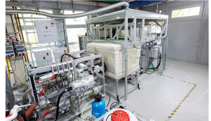
DLR test facility for the investigation of stack units with an EC power of up to 100 kW eI
