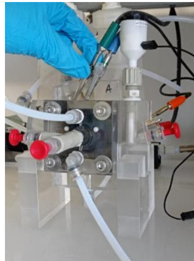
Flow cell for electrochemical characterization (1 cm 2 electrode area)
